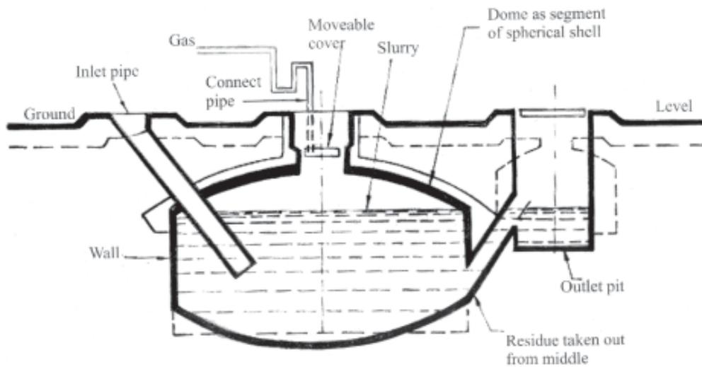
Figure - 2: Fixed Dome Type Biogas - Chinese Model
