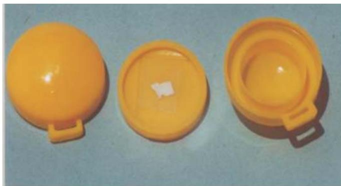
Figure-1: A photograph of the NRPB dosimeter
